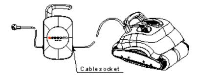
Connect the Control Box to an outside AC power of 100v/240v 50/60Hz with a earth leakage detection device.
