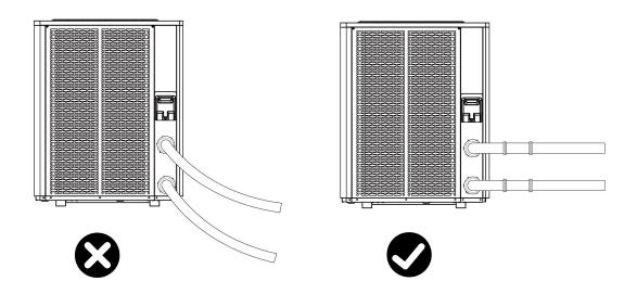
2. In order to guarantee the heating efficiency, the water pipe length should be  $\leq$ 10m between the pool and the heat pump.
