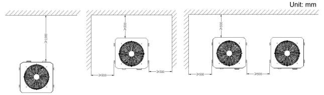
Do not put anything less than one meter in front of the heat pump.
