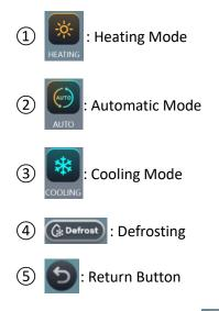
One-Key Defrosting: click " ( , the icon will lights up and does not go out until the unit has finished and exits defrost mode.
